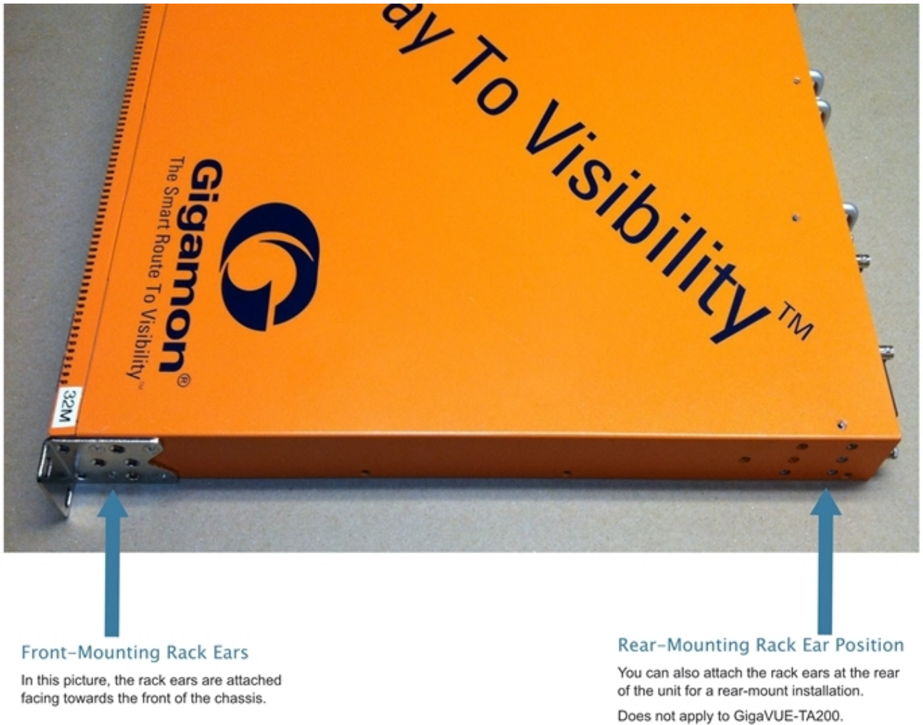
Figure 3 GigaVUE TA Series Traffic Aggregator Rack Ears in Front-Mount Position
